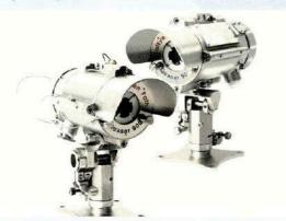
The SafEye Quasar 900 is an open path detection system. It employs "spectral fingerprint" analysis of the atmosphere using the Differential Optical Absorption Spectroscopy (DOAS) technique. With a range from 7m up to 200m the Quasar 900 detects gas hazards in extremely harsh environments where dust, fog, rain, snow or vibration can cause a high reduction of signal.
