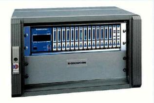
Gasmonitor Plus is a 19" rack based control system for monitoring up to 16 gas detectors or 32 fire zones per rack. Gasmonitor Plus racks can be supplied separately or built into wall mounting or floor standing cabinets and can be engineered into large systems to suit any site requirement. Gas detectors are independently powered and monitored, with a separate gas level display for each.
