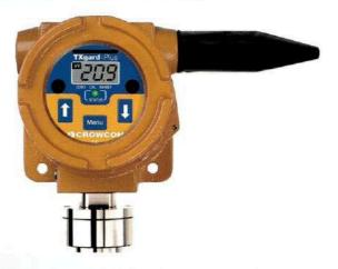
TXgard Plus is a flameproof (Ex d) toxic, or oxygen gas detector with local LCD display. A choice of sensors is available for use in a wide range of applications. Flamgard Plus is a flameproof (Ex d) flammable gas detector with an LCD display. It uses poison resistant pellistors to detect % LEL levels of hydrocarbons, hydrogen and other flammable gases and vapours, including aviation fuel and leaded petrol vapours.
