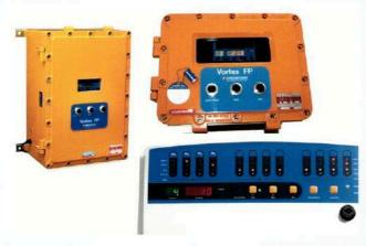
Control panel for monitoring one to twelve gas detectors. Versatile modular system available with up to 32 programmable relays. Includes a gas display, battery back up, internal alarm, one-man calibration feature, RS-485 Modbus communications, event logging and PC software for configuration and monitoring. Available in wall mount, 19" rack, panel mounting or Ex d Flameproof formats.
