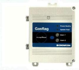
Entry-level control panel for monitoring any 4-20mA flammable, toxic or oxygen gas detector. Includes bright alarm LEDs and a loud sounder. Relays are fitted for switching external devices such as audible / visual alarms or valves. Applications include boiler rooms (flammable gas), swimming pools (chlorine) and vehicle filling stations (LPG/CNG).
