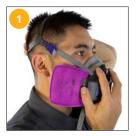
Adjust head cradle, as needed, to fit comfortably on your head. Place the respirator over your mouth and nose, then pull the head harness over the crown of the head.
