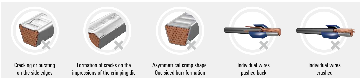
Figure 19: Overview of some crimping errors
