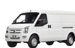
EC 35 DFSK : 1100 kg rated load; 4.8m³ loading space
