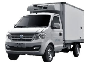
EC 31 Freezer Truck : -20°C to 12°C Freezer, Energy consumption <2.5kw/h
